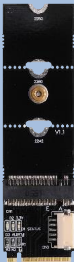
M2E (M.2 Key A Wireless Card to M.2 Key M Adapter) x1
