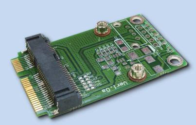
The MM2U-C half to full mini card is a converter tool for minicard interface.
