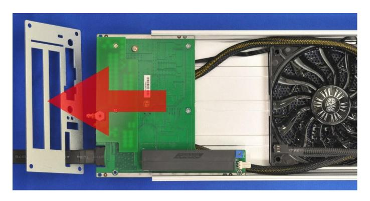
Customers can regulate the speed of fans through R25, R26 which are variable resistors, tips on PCB show you the speed direction.
