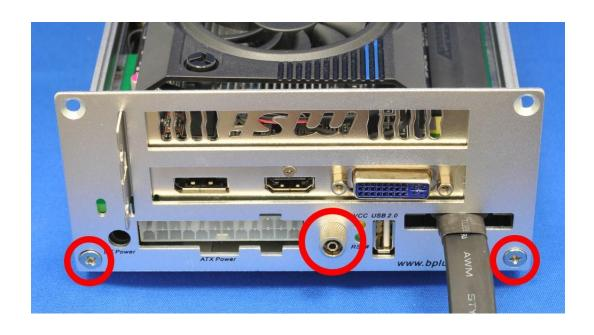
**Step 4: Push PCB module into enclosure:**
