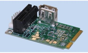
The PCI-E 1x to Mini PCI-E Card 1.0 is a debug tool for PCI-E interface card.
