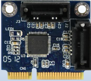
PM362 (SATA to halfmini-PCIE adapter) x1
