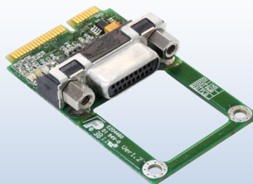
PM3P PCBA (PCB Thickness 1.0mm ) x1
