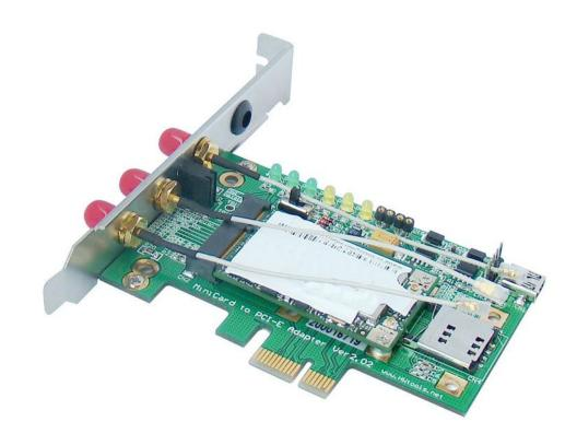
4) Put the wireless antenna on the RP-SMA CONN.
