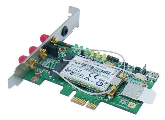
3. Before plug MP2A into PCI-E slot, please ensure cut off the PC power firstly. Then, connect USB cable line or DuPont 5P to 5P cable line ok.
