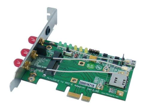
2) Plug mini card device such as wireless LAN card into mini PCI-E connector. The other side should be fixed by two screws.
