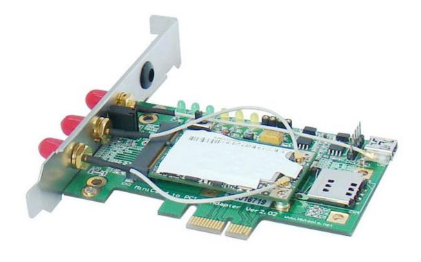
5) Before the user plugs PCI-E connector into PC M/B, please ensure cut off the PC power firstly, then continue plug-in. Finally, please ensure USB cable line or DuPont 5P to 5P cable line connect OK.
