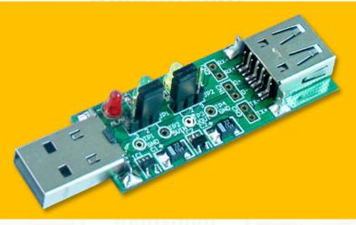
The USB Fixture is a test tool for USB 2.0 / 3.0 interface with multi-functions of voltage swtich, voltage test and current test. It's especially designed to save valuable labor and time in the production environment.
